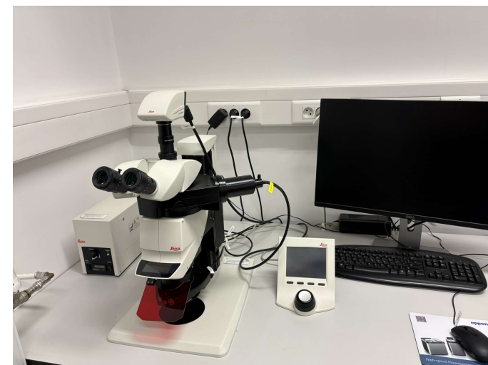
Leica M205 FA fluorescence microscope. The microscope is equipped with a Leica DFC450C camera and GFP LP filters (excitation filter: 480/40 nm; barrier filter: 510/∞ nm), DSR ET filters (excitation filter: 545/30 nm; barrier filter: 620/60 nm)
